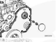
27 mm Remove the crankcase breather and gear retaining nut and washer.
