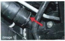
Step 2: Drain the engine coolant by removing the metal retaining clip on the lower radiator line and pulling the line away from the radiator enough to allow the coolant to flow out. As the flow of the coolant slows down and the overflow bottle is empty, reconnect the lower radiator line. (Image 1)
