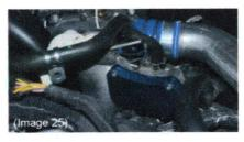
Step 35: Reinstall the intake tube, securing it in place with the two original bolts.
