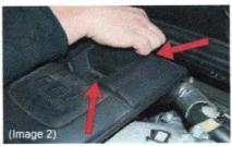
Step 3: Remove the intake resonator that is held in place by two bolts. (Image 2)
